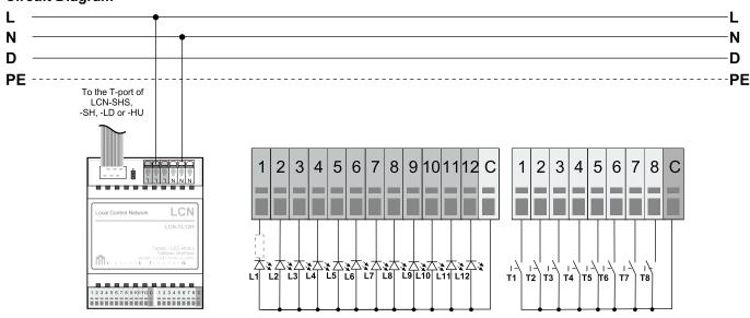
The connecting cables for the switches and LEDs lead N potential!
